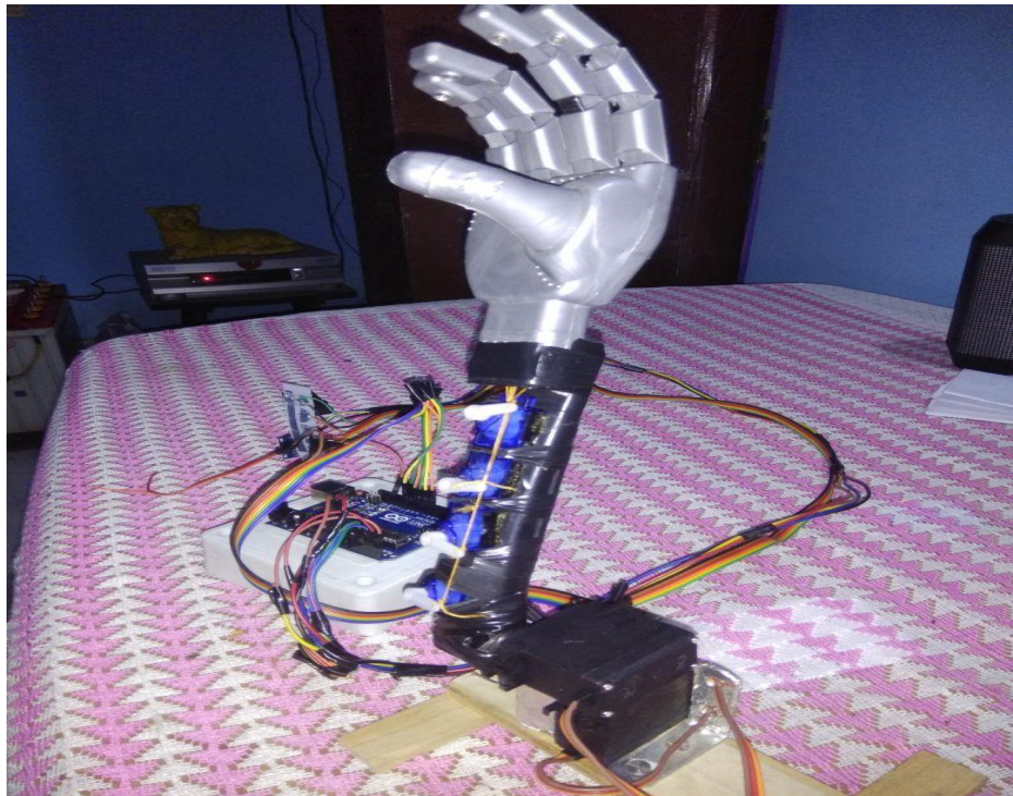
Fig. 4. The working model of the Bionic Arm
